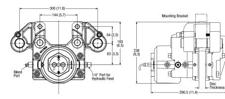
The Twiflex VCS-FL disc brake caliper comprises a single spring module forming the 'active' side of this floating unit and is available for use where space is limited or to accommodate axial disc float of ±6mm (0.24 in).
