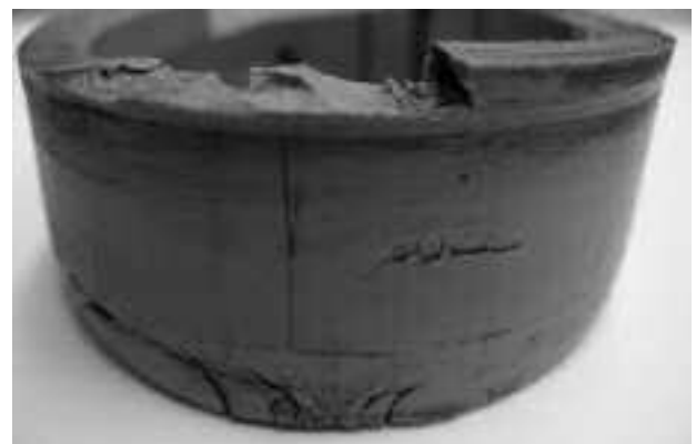
This example indicates that the ThorPlas bearing chamfers were too long and as the bearing was loaded in this area, not enough support was available for the material to take the load. Although the bearing cracked, it did not shatter and remained in one piece.
