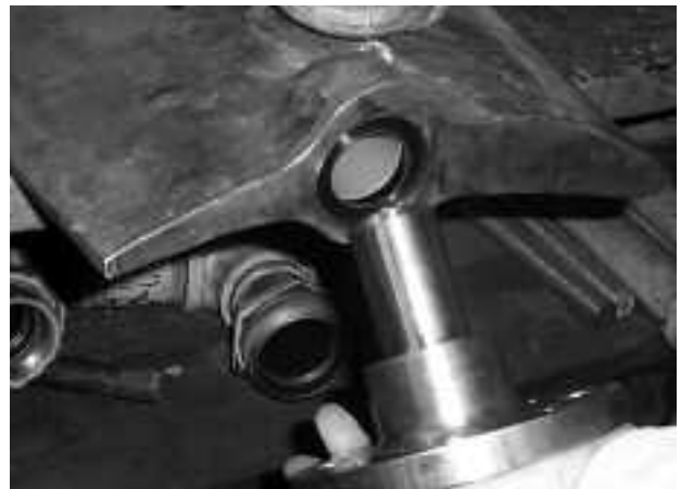
ThorPlas wicket gate bearing with Thorseal
