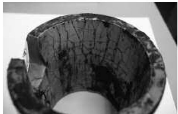
Typical example of ThorPlas bearing with hydrolysis
