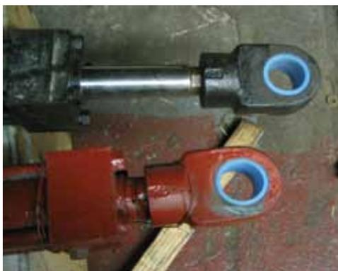
*ThorPlas-Blue steering and linkage bearings installed*
