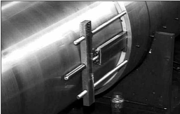
Figure 4: Single Key removal using key extraction tool
