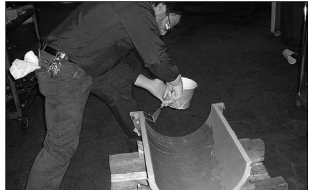
Figure 6: TG-75 being applied to OD of split SXL bearing
