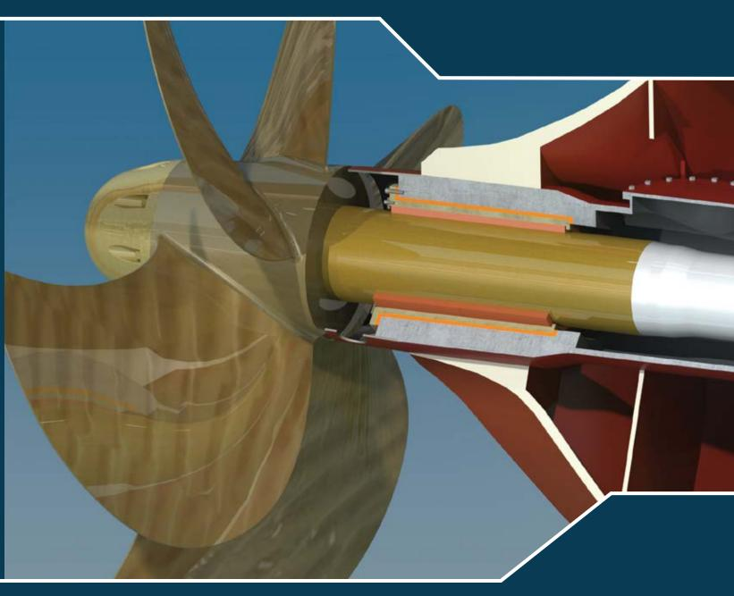
COMPAC SEAWATER LUBRICATED PROPELLER SHAFT BEARING SYSTEM
