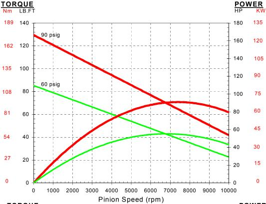
Model: 56K 21 Nozzles 70° F Methane Gas 4.5:1 Gear Ratio
