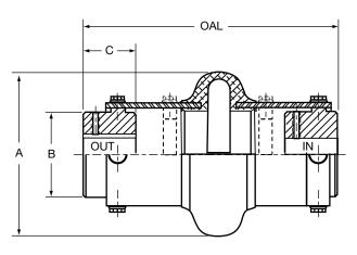
Shaft Spacing from 6.35 mm up to the MAX DBSE can be accommodated by positioning hubs IN or OUT or by using various existing hole patterns. OAL - Over All Length does Not include bolt heads.
