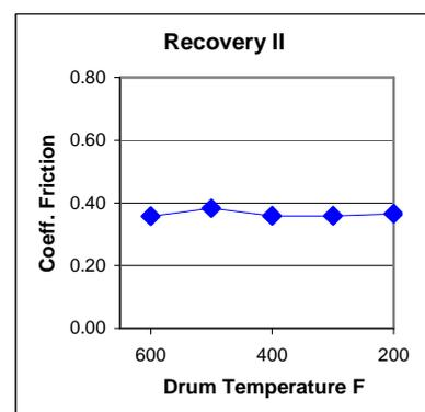
\*Note 1. – Friction values shown are for guide purposes only since values deviate with changes in temperature, pressure and speed. Practical design should include a 25 to 50 percent safety factor.
