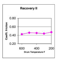
\*Note 1. – Friction values shown are for guide purposes only since values deviate with changes in temperature, pressure and speed. Practical design should include a 25 to 50 percent safety factor.
