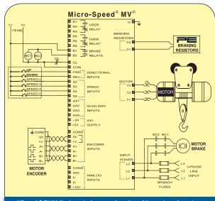
UP and DOWN limit switches can be placed in various locations depending on application requirements. Lights or alarms can be driven by user relays 1 or 2. Two optically isolated analog outputs & serial interface option not shown.
