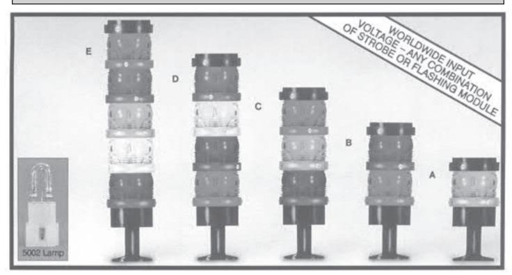
The Model 440 MICROSTACK features multi-color and multiformat optical signalling using strobes and/or steady burning or flashing NEOBE lamps in any combination. NEOBE lamps are gas discharge lamps which have no filament to wear or break. All MICROSTACK modules operate over a worldwide AC input
