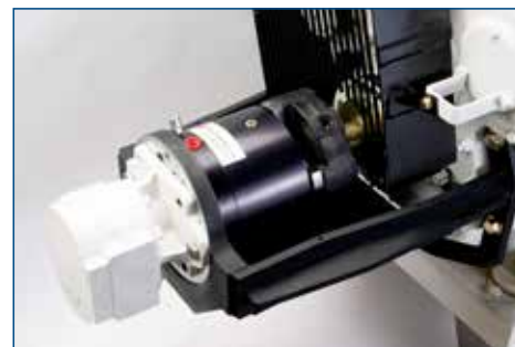
View of front PTO for John Deere 4045T diesel engine
