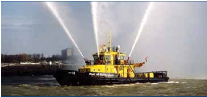
View of typical escort tug equipped with Z-drive propulsion, enabling more maneuverability in congested shipping ports
