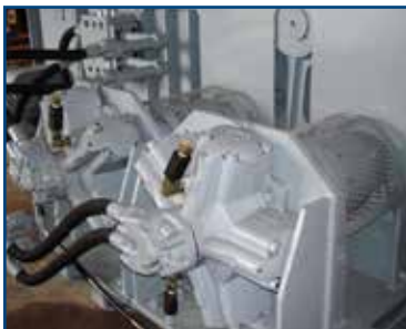
CH clutch mounts between motor and winch
