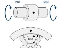
When input torque is reversed, the control member rotates a maximum of 6° to release the opposing set of sprags and then again drives the **output member** through point "B" on these sprags.
