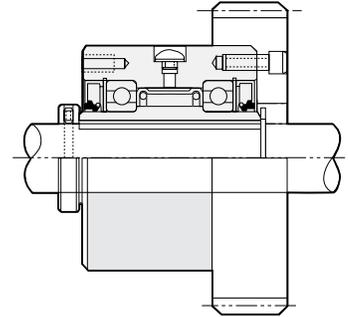
The Model FSO clutches must be axially restrained, see accessories page 122 for set collars, restraint keys and OSHA covers, etc. All fasteners are recommended to be grade 8 bolts.
