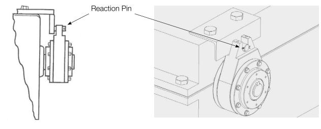
The Model FHB can be axially restrained by a cotter pin in the reaction pin
