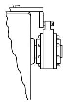
The Model FHB can be axially restrained by a cotter pin in the reaction pin
