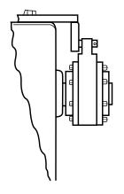
The Model FHB can be axially restrained by a cotter pin in the reaction pin
