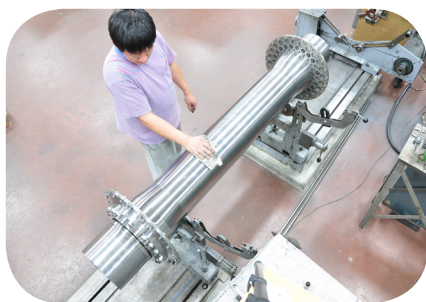
Size 500 FLEXXOR for a centrifugal compressor on the balancing stand
