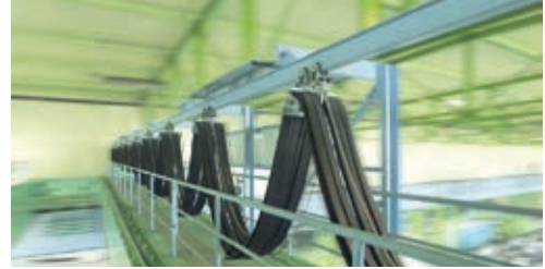
On the go! Program 0350 cable trolley system on a steel mill overhead bridge crane
