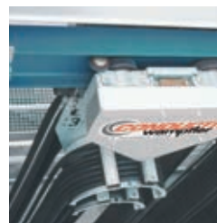
Motorized main cable trolley with magnetic switch for back reach limit stops
