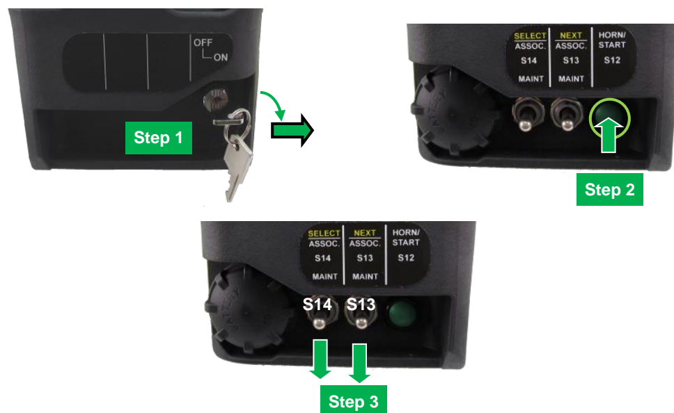
Figure 5. Clearing the ID (Factory Reset)
